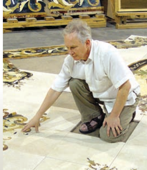
Artist Harri Aalto checks the precision fit of the water-jet-cut stone pieces for one of his custom creations.
